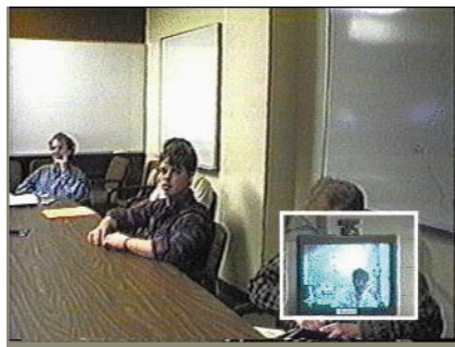
Figure 5. The Virtual Window camera control system in operation. The larger images represent the view received by the remote participant, while the small inset images represent the appearance of the participant on a local video monitor. The motorized camera appears at the top of the video monitor.
