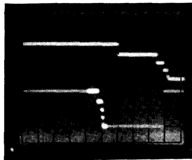
Fig. 8. The output waveform for delay-gate mismatch measurement. The horizontal scales are 50 \text{ ms/div} (lower) and 5 \text{ ms/div} (upper) and the vertical scale is 2 \text{ V/div} .
